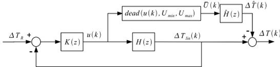
Fig. 3. Resulting feedback-structure when  $H(z) = \hat{H}(z)$ .
